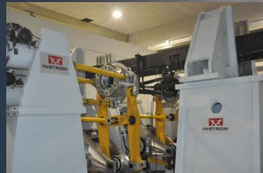
Road load spectrum simulation test
