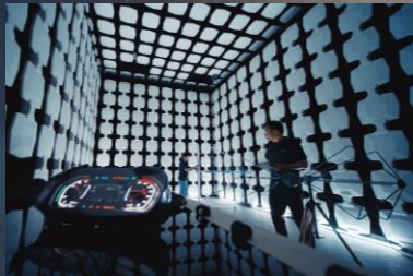
Electromagnetic compatibility test
