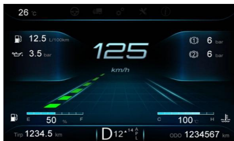
仅检测到左车道线 Only the left lane line detected
