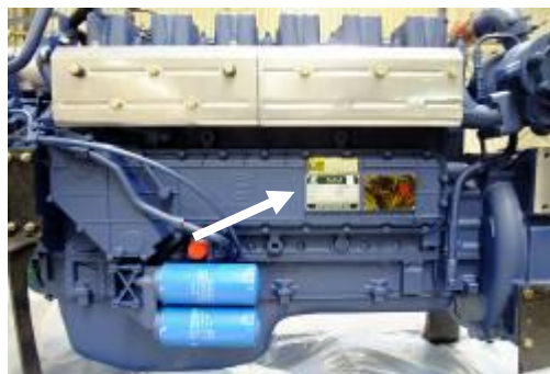
WP10 发动机铭牌位置 Position of WP10 Engine Nameplate
